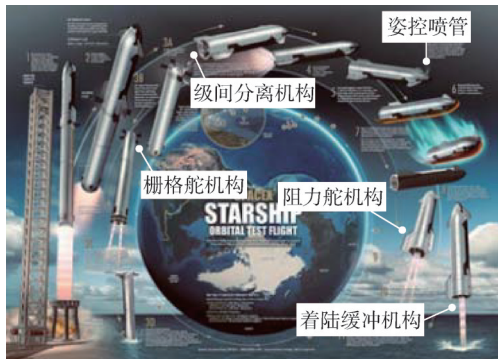
图1 超重-星舰运输系统首次入轨发射飞行任务剖面 Fig.1 Super Heavy-Starship transport system first orbital test flight profile
