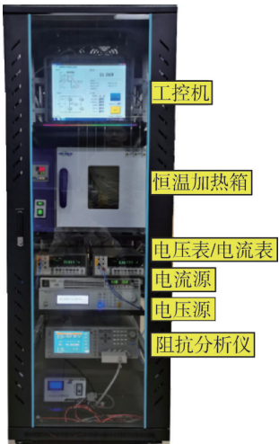
图7 基于直流功率法的PWM波励磁磁心损耗测量平台 Fig.7 Core loss measurement platform under PWM excitation based on DC power method
