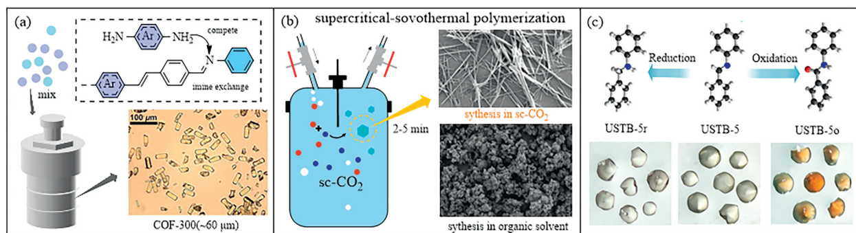
Fig. 8. (a) A modulator was added to the reaction system to decrease the reaction speed and improve the crystal quality. Reproduced with permission [72]. Copyright 2018, the American Association for the Advancement of Science. (b) sc-CO 2 accelerated the reaction process and produced crystals quickly. Reproduced with permission [76]. Copyright 2021, Springer Nature. (c) Linkage changes undergo SCSC transformation. Reproduced with permission [78]. Copyright 2023, Springer Nature.
