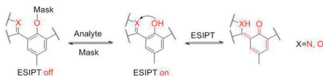
Fig. 2. The design of ESIPT-based probe by masking the hydroxyl group.
