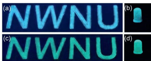
Fig. 5. Color and fluorescence images of characters written by the solution of (a) (1-2-3)_n and (c) (1-2-3)_n + \text{ESY} after irradiation with UV light at 365 nm. Images of the LEDs prepared by coating the solution of (b) (1-2-3)_n and (d) (1-2-3)_n + \text{ESY} .
