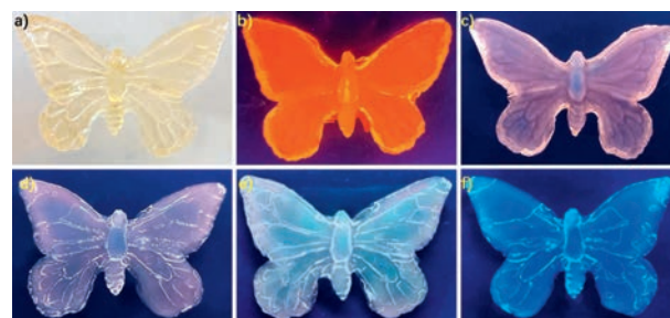
Fig. 6. Photographs of multicolor hydrogels with butterfly pattern under daylight (a) and 365 nm UV light after irradiation with different times (b-f).
