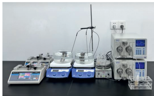
Fig. 6. Continuous-flow synthesis of chiral polysubstituted \gamma -butyrolactones via a dual-enzyme cascade.
