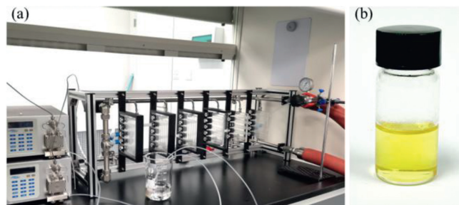
Fig. 3. Scale-up of the continuous-flow system. (a) The setup of 6 parallel microfluidic reactors. (b) The sample of optically pure 3g was obtained as a light yellow liquid.
