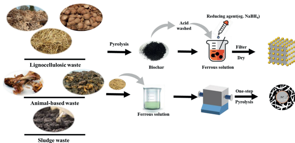
Fig. 2. Two main preparation methods of ZVI-modified biochar.
