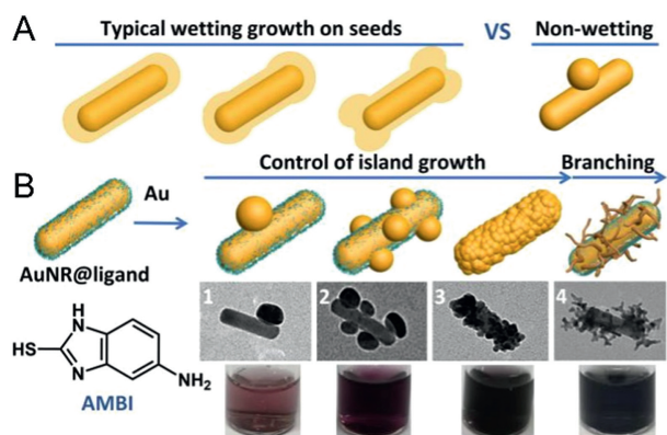
Fig. 3. Schematics illustrating (A) the typical wetting and (B) non-wetting Auon-AuNR homometallic nanostructures, with the corresponding TEM images and photographs. Reproduced with permission [77]. Copyright 2020, Wiley-VCH.
