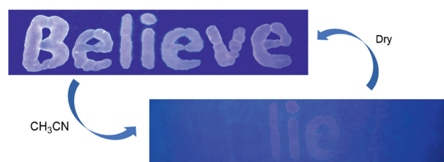
Fig. 6. Information encryption using cages C1 and C2 as the inks.
