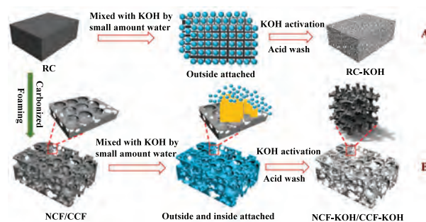
Scheme 1. Schematic diagram of the synthesis route of hierarchical porous carbon (HPC) from coal-based carbon foam (NCF/CCF, route B) with coal (RC, route A) as control.
