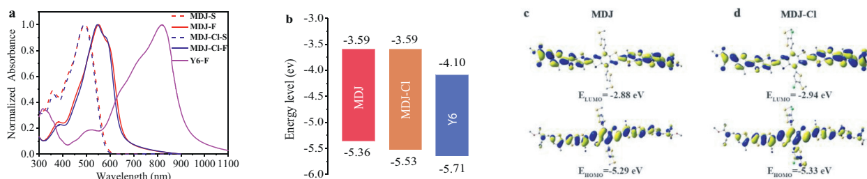
Fig. 2. (a) Normalized absorption spectra of MDJ, MDJ-Cl and Y6 in the \text{CHCl}_3 solution and thin film. (b) Energy level diagram of materials used in the device. Electron density distributions of LUMO and HOMO for (c) MDJ and (d) MDJ-Cl.
