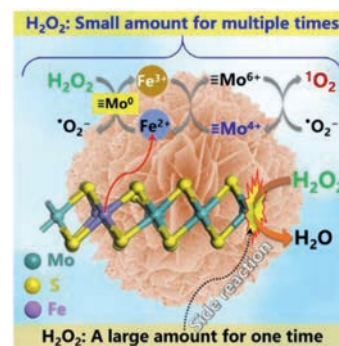
Scheme 1. Possible mechanism of MoS 2 -Fe x for the decomposition of H 2 O 2 in different feeding way.
