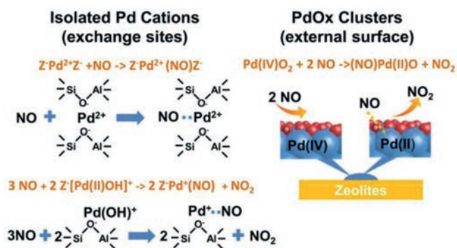
Fig. 3. The interaction of different Pd species with NO. Reprinted with permission [45]. Copyright 2017, American Chemical Society.
