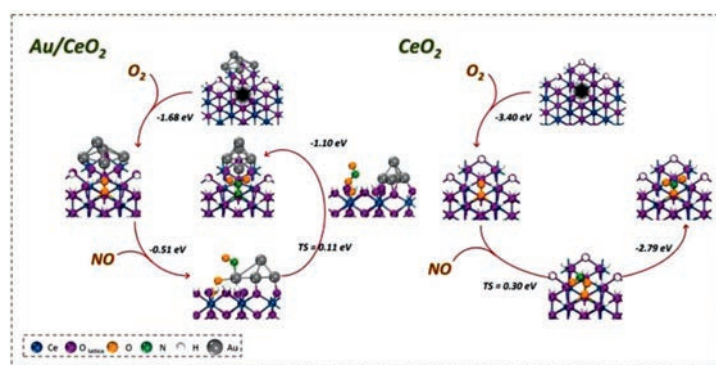
Fig. 19. DFT calculations for NO oxidation on the Au/CeO 2 and CeO 2 with (100) surface exposed. Copied with permission [38]. Copyright 2020, Elsevier.
