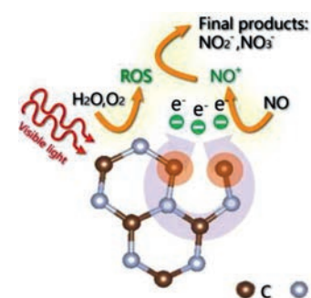
Fig. 20. Illustration of photocatalytic NO removal on N defects sites containing g-C 3 N 4 . Copied with permission [89]. Copyright 2020, Elsevier.
