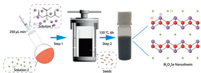
Fig. 1. Schematic diagram of a two-step synthesis process of the \text{Bi}_2\text{O}_2\text{Se} nanosheets.
