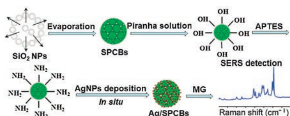
Scheme 1. The schematic diagram of the process for synthesis of Ag/SPCBs and SERS detection of MG.
