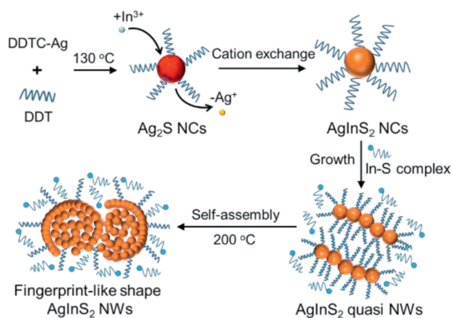
Scheme 1. Schematic illustration showing the morphologies change involved in the synthesis and self-assembly of \text{AgInS}_2 NCs into quasi NWs and fingerprint-like structures.
