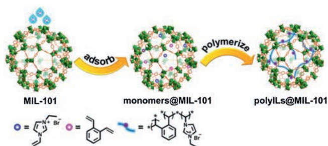
Fig. 2. The preparation of polyILs@MIL-101. Reproduced with permission [21]. Copyright 2018, American Chemical Society.
