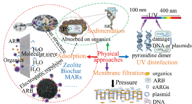
Fig. 2. Removal mechanism of ARGs during the operation of the physical approaches.
