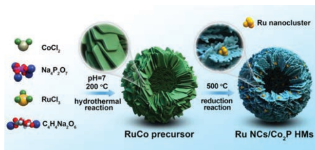
Scheme 1. Schematic illustration of the synthetic procedure for Ru NCs/Co 2 P HMs.
