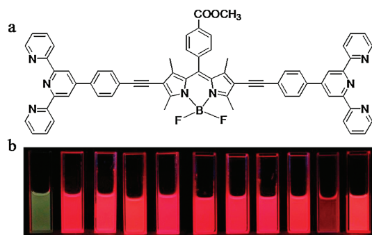
Scheme 1. (a) The chemical structure of BODIPY derivative (BODIPY-DT). (b) The emission colors of BODIPY-DT ( 10^{-5} mol/L) in different organic solvents after staying at room temperature in sunlight for 5 h. From left to right: DMF, DMSO, THF, acetone, p -dimethylbenzene, \text{CH}_2\text{Cl}_2 , methylbenzene, \text{CHCl}_3 , methoxyethanol, acetonitrile, \text{CH}_3\text{COOC}_2\text{H}_5 .
