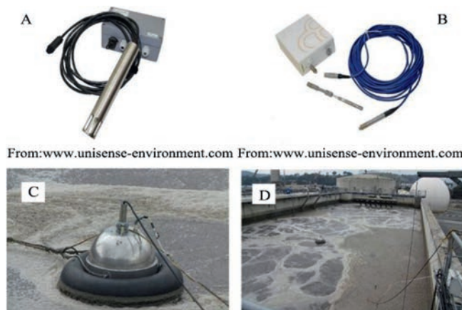
Fig. 2. (A) Full-scale \text{N}_2\text{O} gas sensor and controller box; (B) Full-scale dissolved \text{N}_2\text{O} sensor and controller box; (C) Close-up of gas sensor placed in the sampling hood; (D) Sampling hood placed in full-scale activated sludge SBR. Copied with permission [112]. Copyright 2019, Elsevier.
