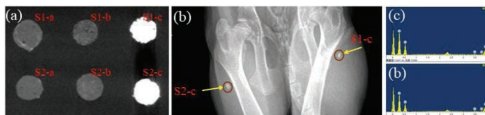
Fig. 3. (a) Micro-CT images of cylinder-shaped samples; (b) In vivo X-ray images of S1-c and S2-c cylinder-shaped samples; (c) EDS image of S1-c; (d) EDS image of S2-c.
