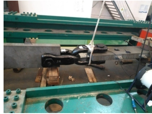
Fig.7 On-site mooring tension monitoring sensor tension test
