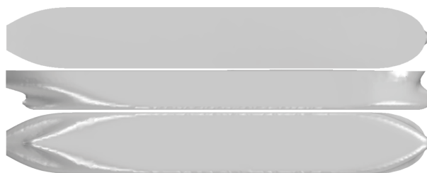
Fig.1 Geometry of the 76 000 DWT ice-strengthened Panamax bulker
