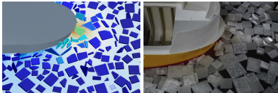
Fig.11 Comparison of local phenomena between model test and numerical simulation ( Fr = 0.077 )
