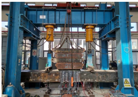
(a) Piled-load loading method
