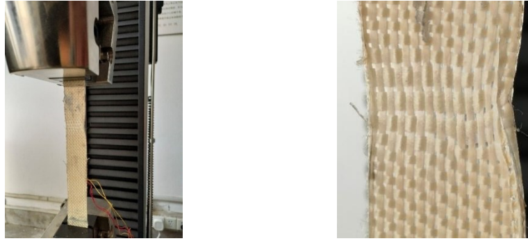
(a) Tensile strength test of bladder skin (b) Failure morphology of bladder skin
