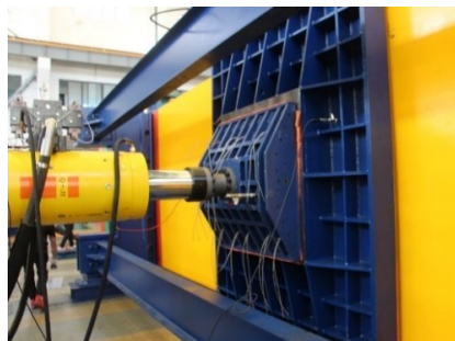
(c) Surface pressure loading system
