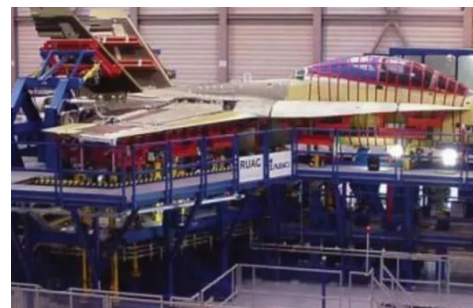
(b) Tension/compression pad loading method
