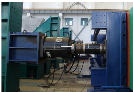
(b) Four-point bending moment loading system
