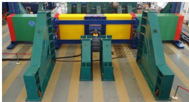
(a) Arrangement of ultimate strength test of box girder
