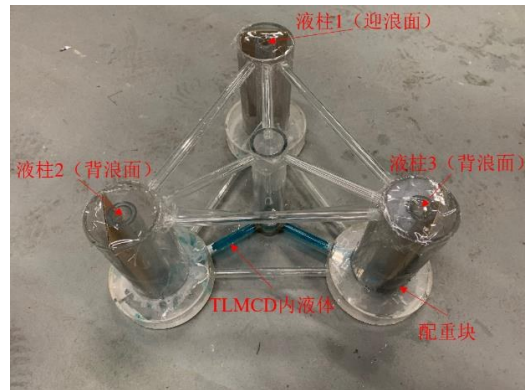
图3 半潜式平台与浮式结构试验模型 Fig.3 Experimental model of semi-submersible platform and TLMCD
