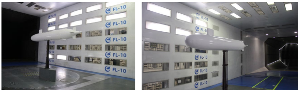
图 6 纯升沉和俯仰运动试验 Fig.6 Pure heave and pitching motion test
