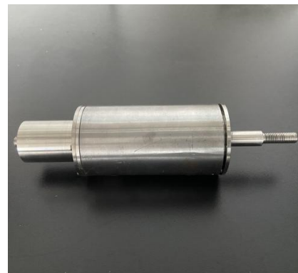
Fig.4 Principle prototype of bidirectional adjustable MRF damper
