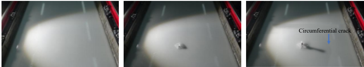
Fig.6 First test (ice length 5000 mm, ice width 2000 mm)
