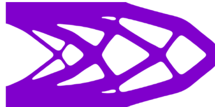
图 7 优化后平面拓扑结构 (算例 1) Fig.7 Plane topology after optimization for Example 1
