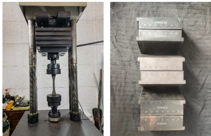
图4 JXG-200 高频疲劳试验机及夹块 Fig.4 JXG-200 high frequency fatigue tester and clamping block
