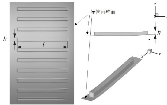
图3 凹槽结构外形参数 Fig.3 Shape and size of the groove
