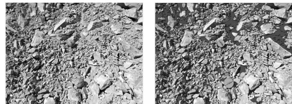
(a) 现场爆破块度照片 (a) Photos of site blasting lumpiness (b) 块度图像法识别效果 (b) The recognition effect of block image method
