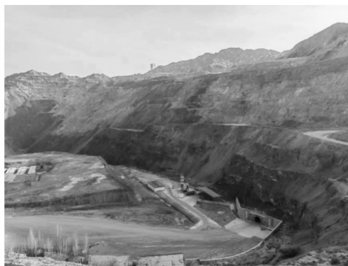
图1 龙首矿露天转地下开采坑底布置图 Fig. 1 Bottom layout diagram of open-pit to underground mining at Longshou Mine
