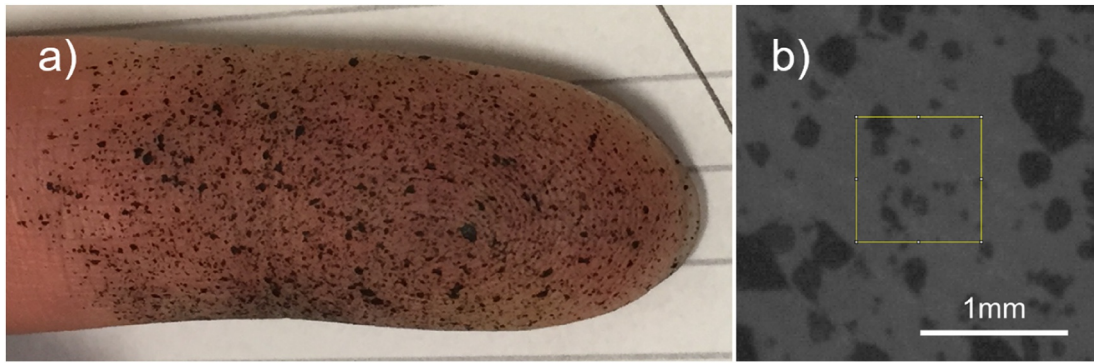
FIGURE 2 | (a) Finger pad with the applied speckles and (b) a magnified image showing an example speckle subset.
