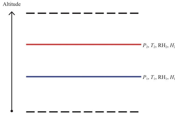
Fig. A1. Schematic showing the stratified structure of atmospheric parameter in calculating the pressure.
