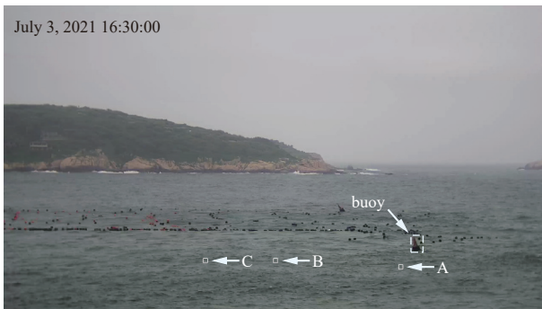
Fig. 6. Frame from the video showing three selected regions (A, B, and C) for wave parameter extraction.
