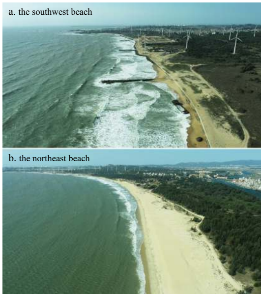
Fig. 7. Observations of beach morphodynamics at Jinghai Bay on February 27, 2023: a. southwest beach with newly-constructed seawalls and groins; b. northeast beach with wide backshore and aeolian dunes.
