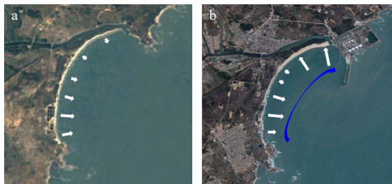
Fig. 8. Conceptual model of shoreline changes due to cross-shore/longshore sediment transport processes observed in this study: Before (a) and after construction of shore-normal structure (b). White arrows represent direction and magnitude of cross-shore sediment transport; blue arrow denotes direction of longshore sediment transport.
