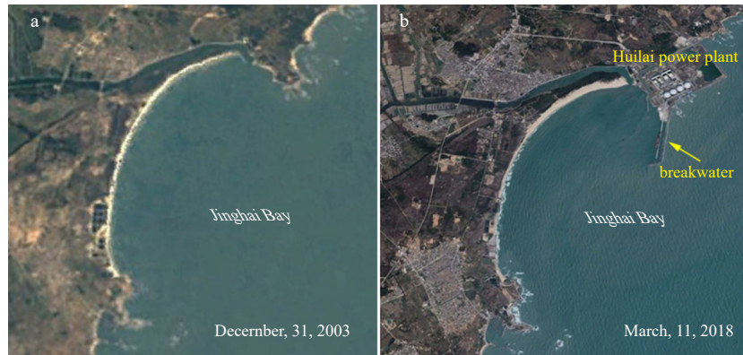
Fig. 2. Planform of Jinghai Bay: Before (a) and after construction of shore-normal breakwater (b).
