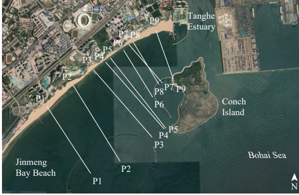
Fig. 4. Sections of beach-profile survey on Jinmeng Bay Beach in August 2021.
