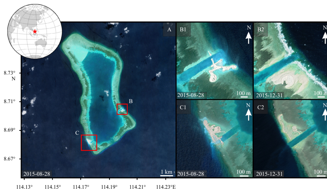
Fig. 1. Destruction of artificial landfill project at Nanhua reef in the South China Sea under the typhoon “Moli”. Satellite imagery are sourced from Google Earth™.
