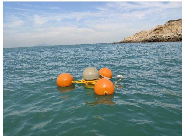
Fig. 1. GPS buoy deployment in the ZW2 campaign. The buoy was moored near the wharf of Zhiwan Island. The TG and the static GPS station were placed on the island.
