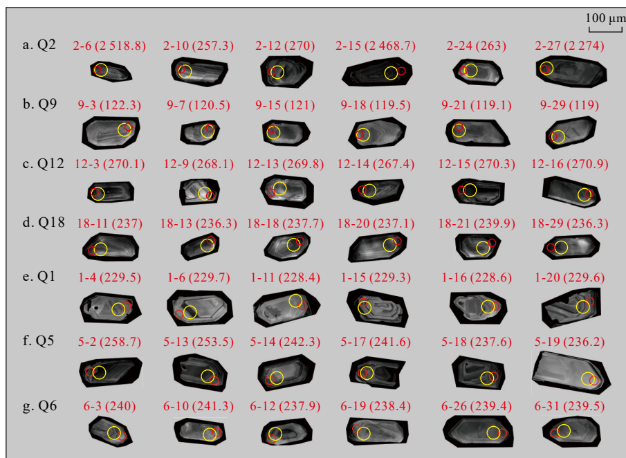
Fig. 2. Cathodoluminescence (CL) images of representative detrital zircons were analyzed for the U-Pb ages. The red and yellow circles denote the analytical spots for the LA-ICP-MS U-Pb dating and Lu-Hf isotopes, respectively. Numbers near the circles indicate are spot number (U-Pb ages), ^{207}\text{Pb}/^{206}\text{Pb} ages are selected for zircons older than 1 000 Ma, and ^{206}\text{Pb}/^{238}\text{U} ages for zircons less than 1 000 Ma.
