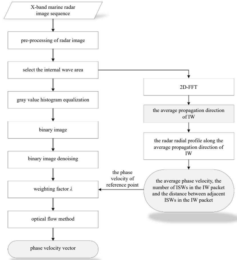
Fig. 3. Retrieval of internal wave (IW) parameters for X-band marine radar images.
