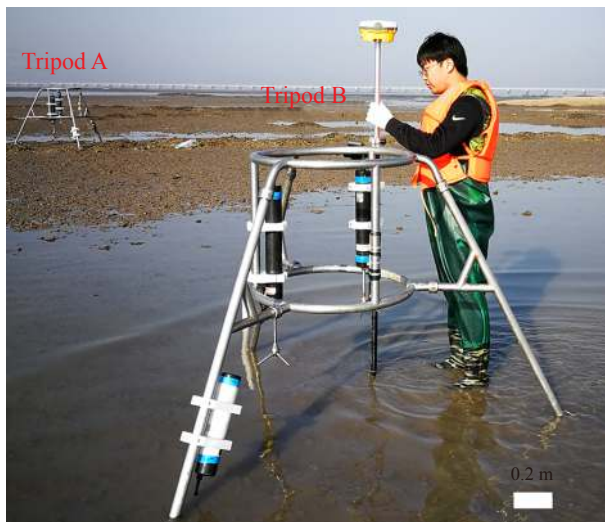
Fig. 2. Tripod observation systems A and B at the reef crest and reef front, respectively.
