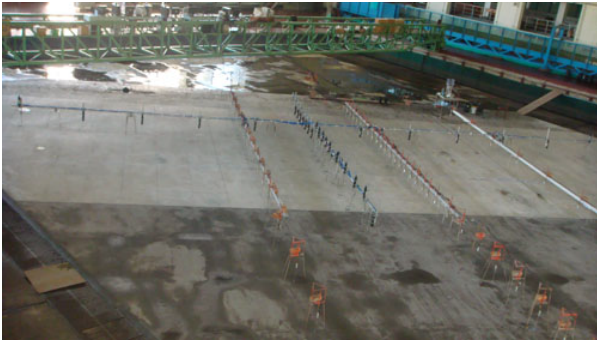
Fig. 6. Experimental photo of layout of velocity meters and wave gauges.
