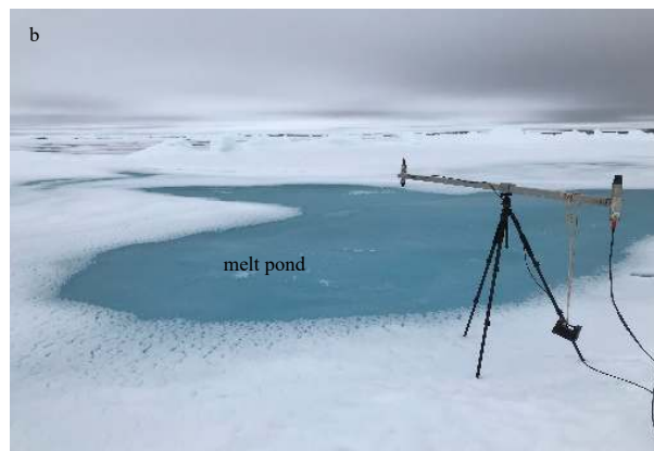
Fig. 3. Schematic diagram of the albedo measurement setup (a) and the photograph of the melt pond (S1) albedo measurement (b).
