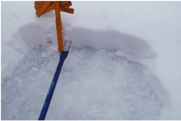
Fig. 2. Snow physical properties measurement by the snow fork.
