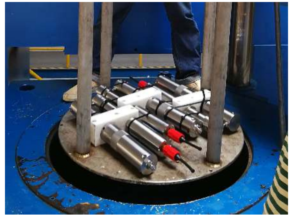
Fig. 9. Water sampling experiment of the samplers in the high-pressure vessel.
